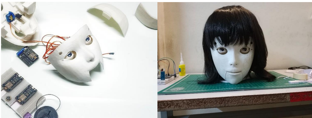
Figure 3: (a) integration of components, (b) final assembly of humanoid robot's head
