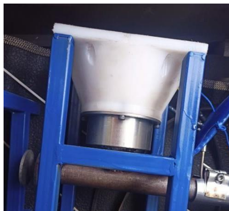
Figure 25 Connectors between shredder and extrusion pipe.
